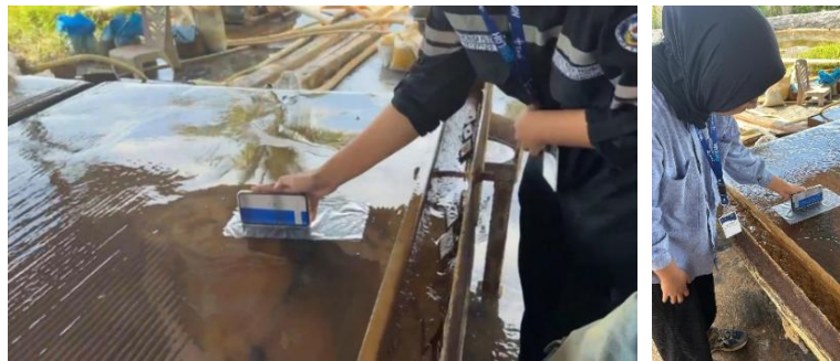
Figure 3. Adjustment and verification of shaking table deck inclination before each experimental run
