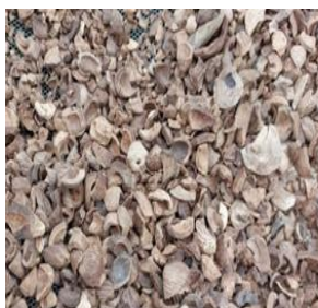
Palm Kernel Shell: washing, drying 110°C and pyrolysis 400°C, 4 hours
