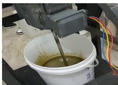
Waste cooking oil filtered, and add the oil to the NaOH solution, add dye and fragrance, then mix
